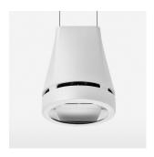
Suspended luminaire with LED, rated life of the LED L80/B10 > 50000 h, chromaticity tolerance 2 SDCM (initial), reflector with oval light distribution pattern, reflector pure aluminium 99,99% in MIRO-Silver®, canopy sheet steel, powder-coated, luminaire head die-cast aluminium, powder-coated, stratowhite
