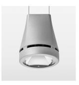
Suspended luminaire with LED, rated life of the LED L80/B10 > 50000 h, chromaticity tolerance 3 SDCM (initial), reflector with circular light distribution pattern, reflector pure aluminium 99,99% in MIRO-Silver®, luminaire head die-cast aluminium, powder-coated, stratosilver, separate driver unit
