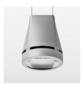
Suspended luminaire with LED, rated life of the LED L80/B10 > 50000 h, chromaticity tolerance 3 SDCM (initial), reflector with oval light distribution pattern, reflector pure aluminium 99,99% in MIRO-Silver®, luminaire head die-cast aluminium, powder-coated, stratosilver, separate driver unit
