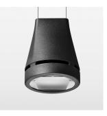
Suspended luminaire with LED, rated life of the LED L80/B10 > 50000 h, colour rendering index CRI > 90, chromaticity tolerance 2 SDCM (initial), reflector with oval light distribution pattern, reflector pure aluminium 99,99% in MIRO-Silver®, luminaire head die-cast aluminium, powder-coated, stratoblack, separate driver unit
