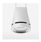
Suspended luminaire with LED, rated life of the LED L80/B10 > 50000 h, colour rendering index CRI > 90, chromaticity tolerance 2 SDCM (initial), reflector with oval light distribution pattern, reflector pure aluminium 99,99% in MIRO-Silver®, luminaire head die-cast aluminium, powder-coated, stratowhite, separate driver unit
