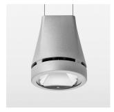
Suspended luminaire with LED, rated life of the LED L80/B10 > 50000 h, chromaticity tolerance 2 SDCM (initial), reflector with circular light distribution pattern, reflector pure aluminium 99,99% in MIRO-Silver®, luminaire head die-cast aluminium, powder-coated, stratosilver, separate driver
