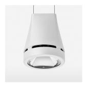
Suspended luminaire with LED, rated life of the LED L80/B10 > 50000 h, chromaticity tolerance 3 SDCM (initial), reflector with circular light distribution pattern, reflector pure aluminium 99,99% in MIRO-Silver®, luminaire head die-cast aluminium, powder-coated, stratowhite, separate driver unit
