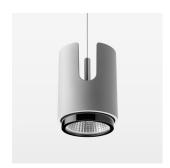
Suspended luminaire with LED, rated life of the LED L80/B10 > 50000 h, chromaticity tolerance 2 SDCM (initial), LED hybrid technology, 3D silicone lens to reduce the proportion of scattered light, reflector with circular light distribution pattern, reflector pure aluminium 99,99% in MIRO-Silver®, segmented and faceted, exchangeable reflector unit in high-sheen black plastic, with glass cover, luminaire housing die-cast aluminium, powder-coated, stratosilver, separate driver unit
