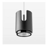
Suspended luminaire with LED, rated life of the LED L80/B10 > 50000 h, chromaticity tolerance 3 SDCM (initial), , reflector with circular light distribution pattern, reflector pure aluminium 99,99% in MIRO-Silver®, segmented and faceted, exchangeable reflector unit in high-sheen black plastic, with glass cover, luminaire housing die-cast aluminium, powder-coated, stratoblack, separate driver unit
