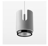
Suspended luminaire with LED, rated life of the LED L80/B10 > 50000 h, chromaticity tolerance 2 SDCM (initial), , reflector with circular light distribution pattern, reflector pure aluminium 99,99% in MIRO-Silver®, segmented and faceted, exchangeable reflector unit in high-sheen black plastic, with glass cover, luminaire housing die-cast aluminium, powder-coated, stratosilver, separate driver unit
