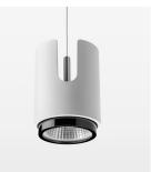
Suspended luminaire with LED, rated life of the LED L80/B10 > 50000 h, colour rendering index CRI > 80, chromaticity tolerance 2 SDCM (initial), , reflector with circular light distribution pattern, reflector pure aluminium 99,99% in MIRO-Silver®, segmented and faceted, exchangeable reflector unit in high-sheen black plastic, with glass cover, luminaire housing die-cast aluminium, powder-coated, stratowhite, separate driver unit
