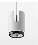
Suspended luminaire with LED, rated life of the LED L80/B10 > 50000 h, chromaticity tolerance 2 SDCM (initial), , reflector with circular light distribution pattern, reflector pure aluminium 99,99% in MIRO-Silver®, segmented and faceted, exchangeable reflector unit in high-sheen black plastic, with glass cover, luminaire housing die-cast aluminium, powder-coated, stratowhite, separate driver unit
