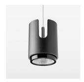
Suspended luminaire with LED, rated life of the LED L80/B10 > 50000 h, colour rendering index CRI > 90, chromaticity tolerance 2 SDCM (initial), LED hybrid technology, 3D silicone lens to reduce the proportion of scattered light, reflector with oval light distribution pattern, reflector pure aluminium 99,99% in MIRO-Silver®, segmented, exchangeable reflector unit in high-sheen black plastic, with glass cover, luminaire housing die-cast aluminium, powder-coated, stratoblack, separate driver unit
