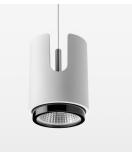
Suspended luminaire with LED, rated life of the LED L80/B10 > 50000 h, colour rendering index CRI > 90, chromaticity tolerance 2 SDCM (initial), LED hybrid technology, 3D silicone lens to reduce the proportion of scattered light, reflector with oval light distribution pattern, reflector pure aluminium 99,99% in MIRO-Silver®, segmented, exchangeable reflector unit in high-sheen black plastic, with glass cover, luminaire housing die-cast aluminium, powder-coated, stratowhite, separate driver unit
