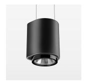
Suspended luminaire with LED, rated life of the LED L80/B10 > 50000 h, chromaticity tolerance 2 SDCM (initial), LED hybrid technology, 3D silicone lens to reduce the proportion of scattered light, reflector with circular light distribution pattern, reflector pure aluminium 99,99% in MIRO-Silver®, segmented and faceted, exchangeable reflector unit in high-sheen black plastic, with glass cover, luminaire housing die-cast aluminium, powder-coated, stratoblack
