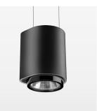
Suspended luminaire with LED, rated life of the LED L80/B10 > 50000 h, chromaticity tolerance 2 SDCM (initial), LED hybrid technology, 3D silicone lens to reduce the proportion of scattered light, reflector with circular light distribution pattern, reflector pure aluminium 99,99% in MIRO-Silver®, segmented and faceted, exchangeable reflector unit in high-sheen black plastic, with glass cover, luminaire housing die-cast aluminium, powder-coated, stratoblack
