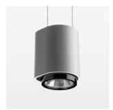
Suspended luminaire with LED, rated life of the LED L80/B10 > 50000 h, chromaticity tolerance 2 SDCM (initial), LED hybrid technology, 3D silicone lens to reduce the proportion of scattered light, reflector with circular light distribution pattern, reflector pure aluminium 99,99% in MIRO-Silver®, segmented and faceted, exchangeable reflector unit in high-sheen black plastic, with glass cover, luminaire housing die-cast aluminium, powder-coated, stratosilver
