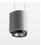
Suspended luminaire with LED, rated life of the LED L80/B10 > 50000 h, colour rendering index CRI > 96, chromaticity tolerance 3 SDCM (initial), LED hybrid technology, 3D silicone lens to reduce the proportion of scattered light, reflector with circular light distribution pattern, reflector pure aluminium 99,99% in MIRO-Silver®, segmented and faceted, exchangeable reflector unit in high-sheen black plastic, with glass cover, luminaire housing die-cast aluminium, powder-coated, stratosilver
