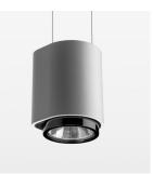
Suspended luminaire with LED, rated life of the LED L80/B10 > 50000 h, chromaticity tolerance 3 SDCM (initial), LED hybrid technology, 3D silicone lens to reduce the proportion of scattered light, reflector with circular light distribution pattern, reflector pure aluminium 99,99% in MIRO-Silver®, segmented and faceted, exchangeable reflector unit in high-sheen black plastic, with glass cover, luminaire housing die-cast aluminium, powder-coated, stratosilver, separate driver unit
