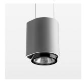
Suspended luminaire with LED, rated life of the LED L80/B10 > 50000 h, chromaticity tolerance 3 SDCM (initial), LED hybrid technology, 3D silicone lens to reduce the proportion of scattered light, reflector with circular light distribution pattern, reflector pure aluminium 99,99% in MIRO-Silver®, segmented and faceted, exchangeable reflector unit in high-sheen black plastic, with glass cover, luminaire housing die-cast aluminium, powder-coated, stratosilver, separate driver unit
