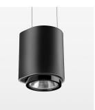
Suspended luminaire with LED, rated life of the LED L80/B10 > 50000 h, chromaticity tolerance 3 SDCM (initial), , reflector with circular light distribution pattern, reflector pure aluminium 99,99% in MIRO-Silver®, segmented and faceted, exchangeable reflector unit in high-sheen black plastic, with glass cover, luminaire housing die-cast aluminium, powder-coated, stratoblack, separate driver unit
