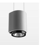
Suspended luminaire with LED, rated life of the LED L80/B10 > 50000 h, colour rendering index CRI > 80, chromaticity tolerance 2 SDCM (initial), , reflector with circular light distribution pattern, reflector pure aluminium 99,99% in MIRO-Silver®, segmented and faceted, exchangeable reflector unit in high-sheen black plastic, with glass cover, luminaire housing die-cast aluminium, powder-coated, stratosilver, separate driver unit
