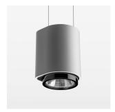
Suspended luminaire with LED, rated life of the LED L80/B10 > 50000 h, colour rendering index CRI > 80, chromaticity tolerance 2 SDCM (initial), , reflector with circular light distribution pattern, reflector pure aluminium 99,99% in MIRO-Silver®, segmented and faceted, exchangeable reflector unit in high-sheen black plastic, with glass cover, luminaire housing die-cast aluminium, powder-coated, stratosilver
