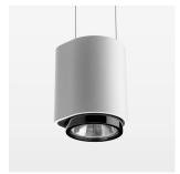
Suspended luminaire with LED, rated life of the LED L80/B10 > 50000 h, colour rendering index CRI > 96, chromaticity tolerance 3 SDCM (initial), , reflector with circular light distribution pattern, reflector pure aluminium 99,99% in MIRO-Silver®, segmented and faceted, exchangeable reflector unit in high-sheen black plastic, with glass cover, luminaire housing die-cast aluminium, powder-coated, stratowhite
