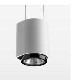
Suspended luminaire with LED, rated life of the LED L80/B10 > 50000 h, chromaticity tolerance 2 SDCM (initial), , reflector with circular light distribution pattern, reflector pure aluminium 99,99% in MIRO-Silver®, segmented and faceted, exchangeable reflector unit in high-sheen black plastic, with glass cover, luminaire housing die-cast aluminium, powder-coated, stratowhite, separate driver unit
