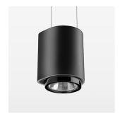
Suspended luminaire with LED, rated life of the LED L80/B10 > 50000 h, colour rendering index CRI > 96, chromaticity tolerance 3 SDCM (initial), LED hybrid technology, 3D silicone lens to reduce the proportion of scattered light, reflector with oval light distribution pattern, reflector pure aluminium 99,99% in MIRO-Silver®, segmented, exchangeable reflector unit in high-sheen black plastic, with glass cover, luminaire housing die-cast aluminium, powder-coated, stratoblack
