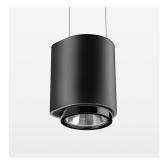
Suspended luminaire with LED, rated life of the LED L80/B10 > 50000 h, colour rendering index CRI > 96, chromaticity tolerance 3 SDCM (initial), LED hybrid technology, 3D silicone lens to reduce the proportion of scattered light, reflector with oval light distribution pattern, reflector pure aluminium 99,99% in MIRO-Silver®, segmented, exchangeable reflector unit in high-sheen black plastic, with glass cover, luminaire housing die-cast aluminium, powder-coated, stratoblack
