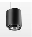
Suspended luminaire with LED, rated life of the LED L80/B10 > 50000 h, chromaticity tolerance 2 SDCM (initial), LED hybrid technology, 3D silicone lens to reduce the proportion of scattered light, reflector with oval light distribution pattern, reflector pure aluminium 99,99% in MIRO-Silver®, segmented, exchangeable reflector unit in high-sheen black plastic, with glass cover, luminaire housing die-cast aluminium, powder-coated, stratoblack
