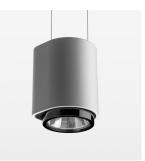
Suspended luminaire with LED, rated life of the LED L80/B10 > 50000 h, colour rendering index CRI > 80, chromaticity tolerance 2 SDCM (initial), LED hybrid technology, 3D silicone lens to reduce the proportion of scattered light, reflector with oval light distribution pattern, reflector pure aluminium 99,99% in MIRO-Silver®, segmented, exchangeable reflector unit in high-sheen black plastic, with glass cover, luminaire housing die-cast aluminium, powder-coated, stratosilver, separate driver unit
