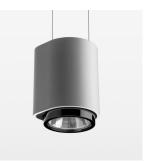
Suspended luminaire with LED, rated life of the LED L80/B10 > 50000 h, colour rendering index CRI > 80, chromaticity tolerance 2 SDCM (initial), LED hybrid technology, 3D silicone lens to reduce the proportion of scattered light, reflector with oval light distribution pattern, reflector pure aluminium 99,99% in MIRO-Silver®, segmented, exchangeable reflector unit in high-sheen black plastic, with glass cover, luminaire housing die-cast aluminium, powder-coated, stratosilver
