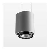
Suspended luminaire with LED, rated life of the LED L80/B10 > 50000 h, chromaticity tolerance 2 SDCM (initial), LED hybrid technology, 3D silicone lens to reduce the proportion of scattered light, reflector with oval light distribution pattern, reflector pure aluminium 99,99% in MIRO-Silver®, segmented, exchangeable reflector unit in high-sheen black plastic, with glass cover, luminaire housing die-cast aluminium, powder-coated, stratosilver, separate driver unit
