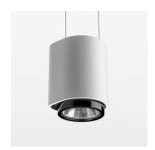
Suspended luminaire with LED, rated life of the LED L80/B10 > 50000 h, colour rendering index CRI > 80, chromaticity tolerance 2 SDCM (initial), LED hybrid technology, 3D silicone lens to reduce the proportion of scattered light, reflector with oval light distribution pattern, reflector pure aluminium 99,99% in MIRO-Silver®, segmented, exchangeable reflector unit in high-sheen black plastic, with glass cover, luminaire housing die-cast aluminium, powder-coated, stratowhite, separate driver unit
