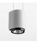
Suspended luminaire with LED, rated life of the LED L80/B10 > 50000 h, chromaticity tolerance 2 SDCM (initial), LED hybrid technology, 3D silicone lens to reduce the proportion of scattered light, reflector with oval light distribution pattern, reflector pure aluminium 99,99% in MIRO-Silver®, segmented, exchangeable reflector unit in high-sheen black plastic, with glass cover, luminaire housing die-cast aluminium, powder-coated, stratowhite
