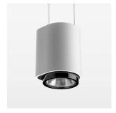
Suspended luminaire with LED, rated life of the LED L80/B10 > 50000 h, chromaticity tolerance 3 SDCM (initial), LED hybrid technology, 3D silicone lens to reduce the proportion of scattered light, reflector with oval light distribution pattern, reflector pure aluminium 99,99% in MIRO-Silver®, segmented, exchangeable reflector unit in high-sheen black plastic, with glass cover, luminaire housing die-cast aluminium, powder-coated, stratowhite, separate driver unit
