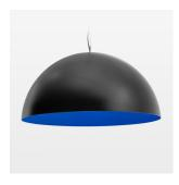
Decorative suspended luminaire with hub holder E27, max 150W, shade made of painted aluminium, black / traffic blue, metal trim ring (diameter 95mm) around hub holder, 28 ventilation openings (diameter 5mm) conzentric circular arrangement, double-isulated cabling, clampingdevice on cable ends if feed cable > 80 mm, power feed cable and canopy black, steel cable hanging set, ceiling-mounting, 1.5m cable
