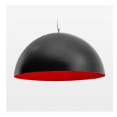
Decorative suspended luminaire with hub holder E27, max 150W, shade made of painted aluminium, black / traffic red, metal trim ring (diameter 95mm) around hub holder, 28 ventilation openings (diameter 5mm) conzentric circular arrangement, double-isulated cabling, clampingdevice on cable ends if feed cable > 80 mm, power feed cable and canopy black, steel cable hanging set, ceiling-mounting, 3m cable
