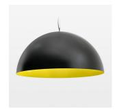
Decorative suspended luminaire with hub holder E27, max 150W, shade made of painted aluminium, black / traffic yellow, metal trim ring (diameter 95mm) around hub holder, 28 ventilation openings (diameter 5mm) conzentric circular arrangement, double-isulated cabling, clampingdevice on cable ends if feed cable > 80 mm, power feed cable and canopy black, steel cable hanging set, ceiling-mounting, 6m cable
