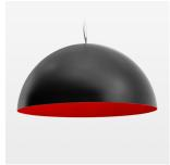
Decorative suspended luminaire with hub holder E27, max 150W, shade made of painted aluminium, black / traffic red, metal trim ring (diameter 95mm) around hub holder, 28 ventilation openings (diameter 5mm) conzentric circular arrangement, double-isulated cabling, clampingdevice on cable ends if feed cable > 80 mm, power feed cable and canopy black, steel cable hanging set, ceiling-mounting, 6m cable
