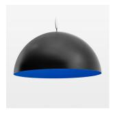
Decorative suspended luminaire with hub holder E27, max 150W, shade made of painted aluminium, black / traffic blue, metal trim ring (diameter 95mm) around hub holder, 28 ventilation openings (diameter 5mm) conzentric circular arrangement, double-isulated cabling, clampingdevice on cable ends if feed cable > 80 mm, power feed cable and canopy black, steel cable hanging set, multiadapter, 1.5m cable
