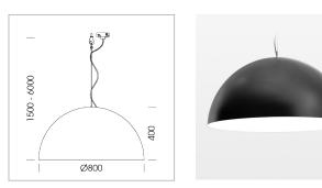
Decorative suspended luminaire with hub holder E27, max 150W, shade made of painted aluminium, black / pure white, metal trim ring (diameter 95mm) around hub holder, 28 ventilation openings (diameter 5mm) conzentric circular arrangement, double-isulated cabling, clampingdevice on cable ends if feed cable > 80 mm, power feed cable and canopy black, steel cable hanging set, multiadapter, 1.5m cable
