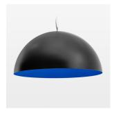
Decorative suspended luminaire with hub holder E27, max 150W, shade made of painted aluminium, black / traffic blue, metal trim ring (diameter 95mm) around hub holder, 28 ventilation openings (diameter 5mm) conzentric circular arrangement, double-isulated cabling, clampingdevice on cable ends if feed cable > 80 mm, power feed cable and canopy black, steel cable hanging set, multiadapter, 3m cable
