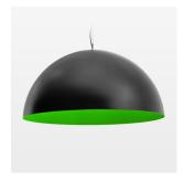
Decorative suspended luminaire with hub holder E27, max 150W, shade made of painted aluminium, black / yellow-green, metal trim ring (diameter 95mm) around hub holder, 28 ventilation openings (diameter 5mm) conzentric circular arrangement, double-isulated cabling, clampingdevice on cable ends if feed cable > 80 mm, power feed cable and canopy black, steel cable hanging set, multiadapter, 3m cable
