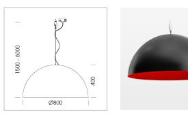
Decorative suspended luminaire with hub holder E27, max 150W, shade made of painted aluminium, black / traffic red, metal trim ring (diameter 95mm) around hub holder, 28 ventilation openings (diameter 5mm) conzentric circular arrangement, double-isulated cabling, clampingdevice on cable ends if feed cable > 80 mm, power feed cable and canopy black, steel cable hanging set, multiadapter, 3m cable
