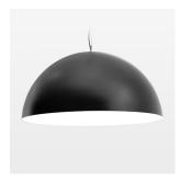
Decorative suspended luminaire with hub holder E27, max 150W, shade made of painted aluminium, black / pure white, metal trim ring (diameter 95mm) around hub holder, 28 ventilation openings (diameter 5mm) conzentric circular arrangement, double-isulated cabling, clampingdevice on cable ends if feed cable > 80 mm, power feed cable and canopy black, steel cable hanging set, multiadapter, 3m cable
