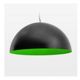
Decorative suspended luminaire with hub holder E27, max 150W, shade made of painted aluminium, black / yellow-green, metal trim ring (diameter 95mm) around hub holder, 28 ventilation openings (diameter 5mm) conzentric circular arrangement, double-isulated cabling, clampingdevice on cable ends if feed cable > 80 mm, power feed cable and canopy black, steel cable hanging set, multiadapter, 6m cable
