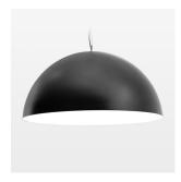
Decorative suspended luminaire with hub holder E27, max 150W, shade made of painted aluminium, black / pure white, metal trim ring (diameter 95mm) around hub holder, 28 ventilation openings (diameter 5mm) conzentric circular arrangement, double-isulated cabling, clampingdevice on cable ends if feed cable > 80 mm, power feed cable and canopy black, steel cable hanging set, multiadapter, 6m cable
