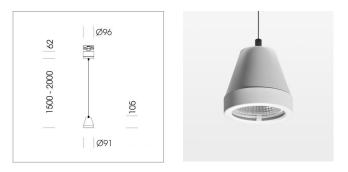
Suspended luminaire with LED, rated life of the LED L80/B10 > 50000 h, colour rendering index CRI > 96, chromaticity tolerance 3 SDCM (initial), reflector with circular light distribution pattern, reflector pure aluminium 99,99% in MIRO-Silver®,segmented and faceted, 3D lens silicon to reduce the proportion of scattered light, luminaire head die-cast aluminium, powdercoated, stratowhite
