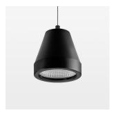
Suspended luminaire with LED, rated life of the LED L80/B10 > 50000 h, colour rendering index CRI > 80, chromaticity tolerance 2 SDCM (initial), reflector with circular light distribution pattern, reflector pure aluminium 99,99% in MIRO-Silver®, segmented and faceted, luminaire head die-cast aluminium, powder-coated, stratoblack
