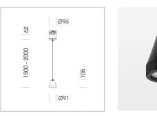
Suspended luminaire with LED, rated life of the LED L80/B10 > 50000 h, colour rendering index CRI > 80, chromaticity tolerance 2 SDCM (initial), reflector with circular light distribution pattern, reflector pure aluminium 99,99% in MIRO-Silver®,segmented and faceted, luminaire head die-cast aluminium, powder-coated, stratoblack
