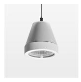
Suspended luminaire with LED, rated life of the LED L80/B10 > 50000 h, colour rendering index CRI > 80, chromaticity tolerance 2 SDCM (initial), reflector with circular light distribution pattern, reflector pure aluminium 99,99% in MIRO-Silver®, segmented and faceted, luminaire head die-cast aluminium, powder-coated, stratowhite
